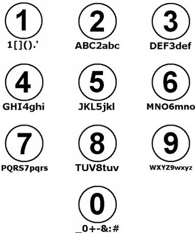
Entering text data is done by pressing keys multiple times to show the character required. The display will change as the key is pressed. Using the character key map shown, to enter the name John, the ⑤ key is pressed once move the cursor one location to the right with the ► key. Press the ⑥ key seven times and repeat the procedure for the other characters in the text entry.
