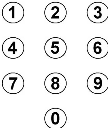
Numerical keys from 0 to 9 are used to enter your User Code to logon to the Protégé LCD Keypad. When in a scroll display the ① key scrolls the display up and the ③ key scrolls down. When controlling devices the ① key turns the device on, ② key turns the device off and the ③ key will latch the device in the on state.
