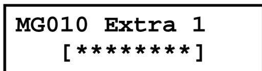
The display will show the option entry screen for the first extra menus that the menu group will allow access to. An option can be toggled on and off by using the numerical keys ① to ⑧. To view the options in text entry mode press the
