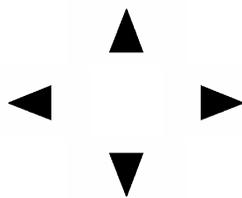
Arrow keys are located on the navigation pad and are used to scroll the menu, move the focus of a program window to the next screen and move the cursor when programming or editing values.
