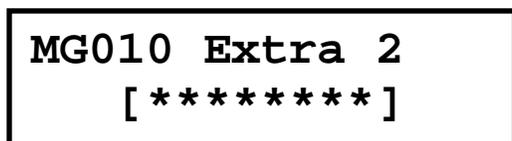
The display will show the option entry screen for the second extra menus that the menu group will allow access to. An option can be toggled on and off by using the numerical keys ① to ⑧. To view the options in text entry mode press the
